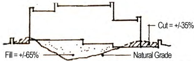
ACCEPTABLE LOW CENTER SITE - TERRACED FLOOR LEVELS
